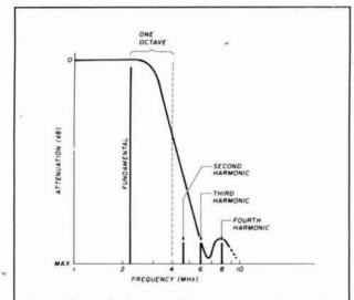
fig. 1. How a half-octave filter attenuates harmonics. Since harmonics are located at least one octave away from any fundamental, a worst case analysis for the entire range of 2 to 30 MHz indicates that several contiguous filters covering half-octaves will reject harmonics always by the same amount. An automatic switched bank of eight half half-octave filters are required to cover the 2 to 30 MHz range.
